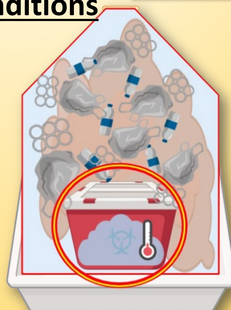
Figure 3. Sharps Container Microclimate Challenge Sealed containers trap cool air, preventing steam penetration and sterilization.
